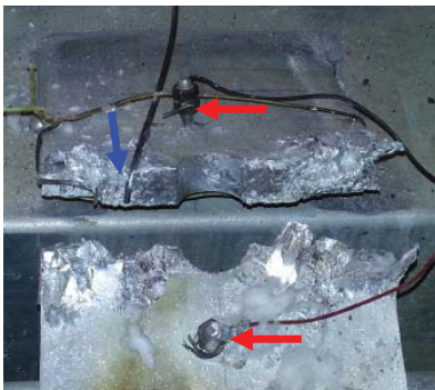
Figure 7. Welded fuse on an EMAL Potline 3 pot after breaking. Red arrows show voltage probes, blue arrow shows the thermocouple.
