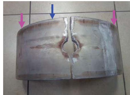
Figure 5. Clamped fuse after the trial, with indication of the position of voltage probes (pink arrows on the sides) and of the thermocouple (blue arrow in the middle).
