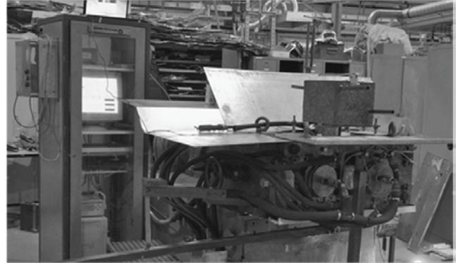
Figure 1. Twin-roll caster used for the manufacturing the aluminium strips.
