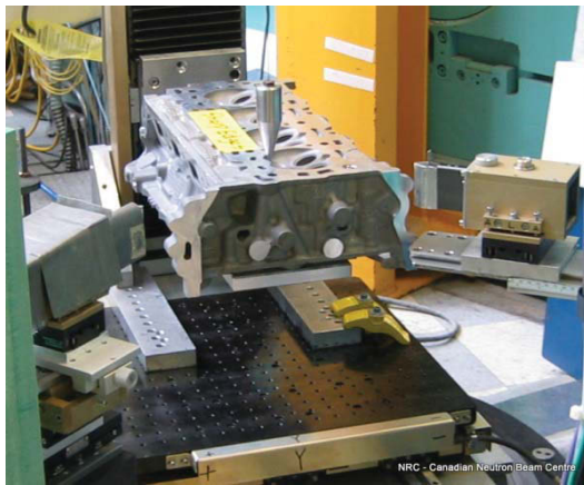
Figure 2. Cylinder head setup at L3. Longitudinal orientation of the engine head corresponds to the "hoop" orientation of the I-E valve bridge.
