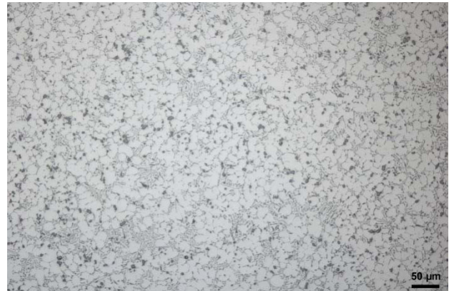
Figure 6: Specimen of a die casting plate with fine, evenly distributed primary Al-Fe-Mn phases. This - through chill casting determined - promising alloy shows optimal Fe/Mn results and was cast with process parameters suitable for series production of crash relevant parts.
