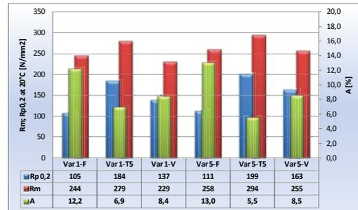
Figure 4. Mechanical properties of the AlSi8.5-alloy (conventional [Var. 1] and optimised alloy [Var. 5]; F=as cast; T5=180°C/2,5h; V=180°C/120h)
