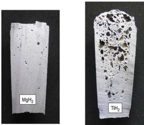
Figure 10. Examples of aluminium foam structures using MgH<sub>2</sub> and TiH<sub>2</sub>.
