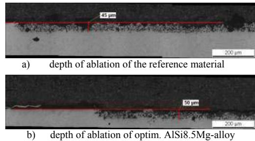
Figure 5. Comparison of the corrosion behavior
