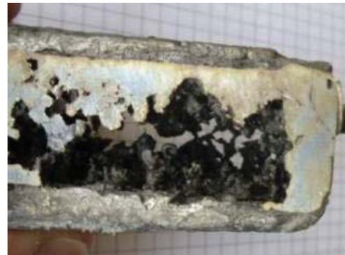
Figure 9. Resulting aluminium structure after dissolving the grains of salt.
