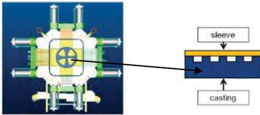
Figure 6. Die casting mould with four sliders which forms a one side formation of the cooling channels. (right: enlarged section of the outside area of the stator)
