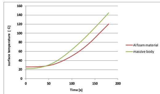
Figure 11. Comparative temperature measurement between a sample made of aluminium foam sandwich and a massive body sample
