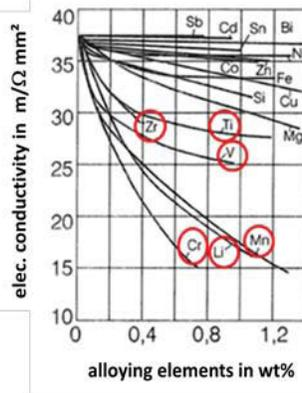
Figure 2. Influence of the alloying elements on the Electrical conductivity, [4].
