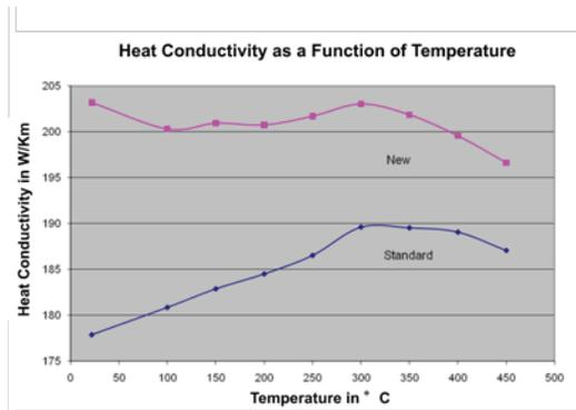
Figure 3. Potential of the boron treatment for the heat conductivity improvement (AlSi7Mg), [5].
