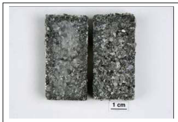
Fig.2. Bauxite brick sample cross section after testing at 850°C/ 96h. No visible infiltration & cracks
