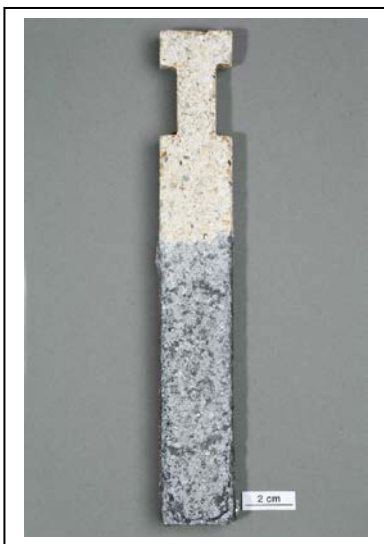
Fig.7. Bauxite brick finger after Al-immersion test
