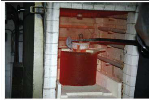
Fig.5. Silicon carbide crucible during the alkali salt input. Fig 6. Retainer with 5 fingers after 48 h. end of test
