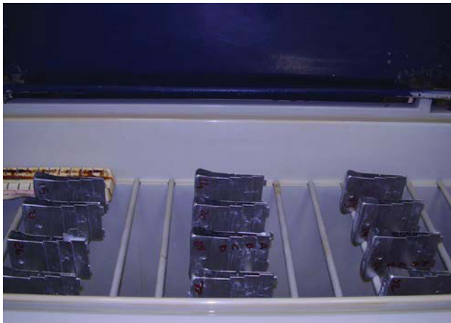
Figure 11. Set-up of the corrosion batch for the experiment
