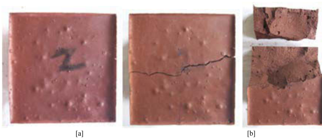
Figure 7. Sample (a) before and (b) after 20 freezing-thawing cycles
