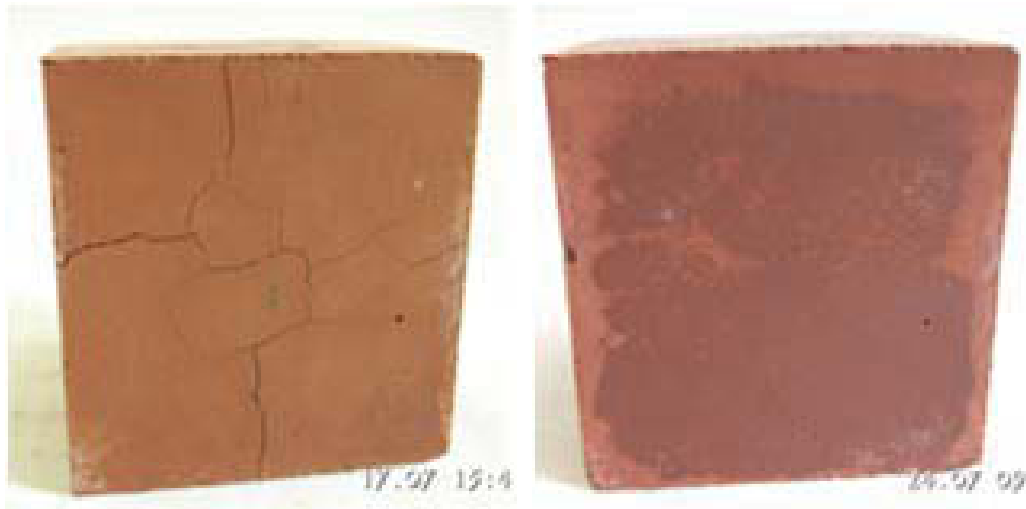
Figure 5. Specimen after curing at 80°C for 3 hours (left) and 7 days (right)
