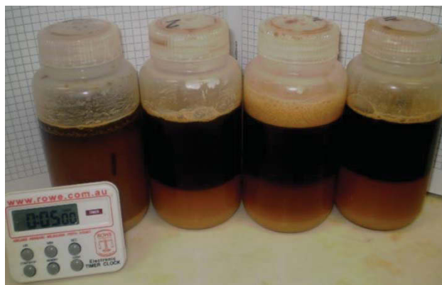
Figure 3. Foam formation 5 minutes after agitation of slurries Left to right: Undosed slurry (no CGM treatment), CGMax (B), Conventional CGM 1, Conventional CGM 2.
