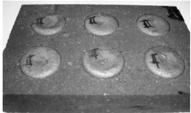
Figure 1. Anode carbon mold with cast iron test specimens.
