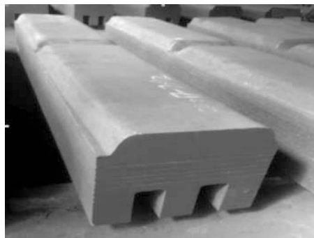
Figure 4: The typical cathode with grooves
