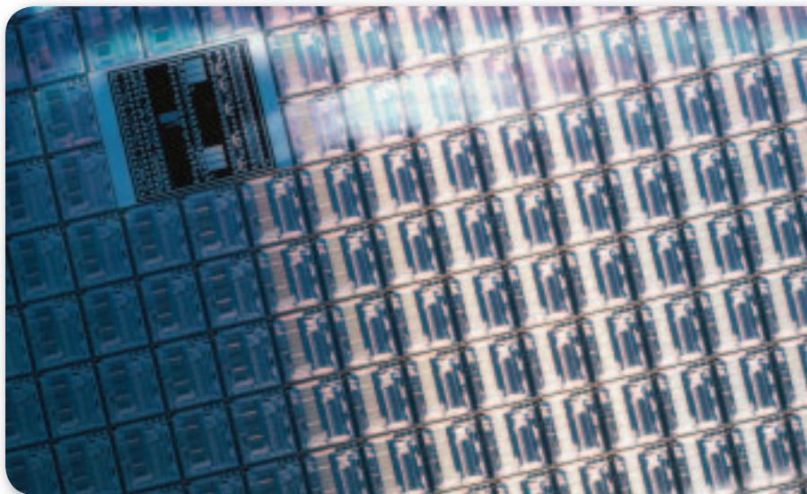
■ Figure 15.16 Sulfur hexafluoride is used to etch minute and sometimes intricate patterns on silicon wafers in the production of semiconductor devices. Semiconductors are important components of modern electronic equipment, including computers, cell phones, and MP3 players.
