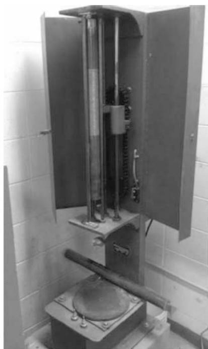
Figure 2. Apparatus used for the compaction of ramming paste: Proctor Mechanical Rammer
