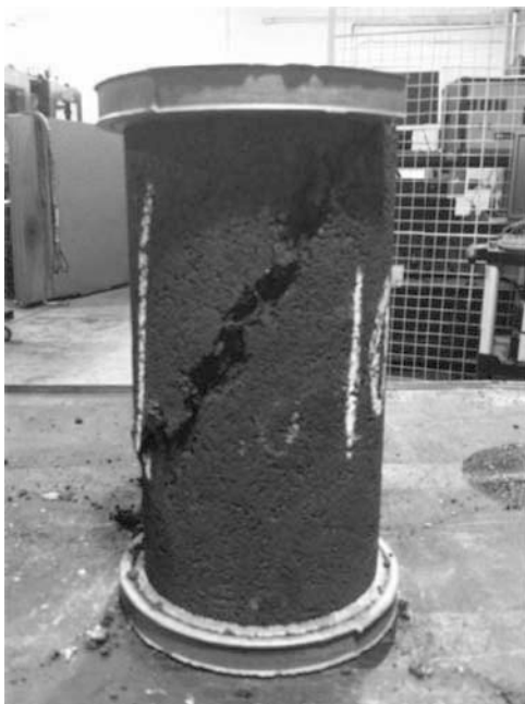
Figure 15. Typical rupture of the baked samples
