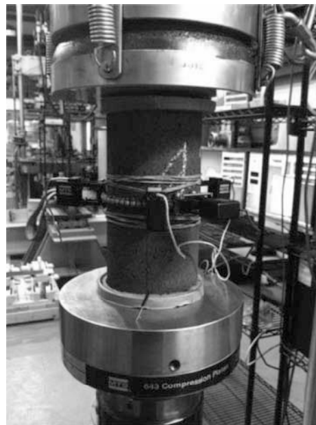
Figure 3. Layout of the sample during compression tests
