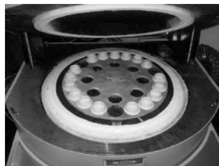
Figure 13: “Equi-Distance” sample placement represented by the dark, nichrome crucibles.
