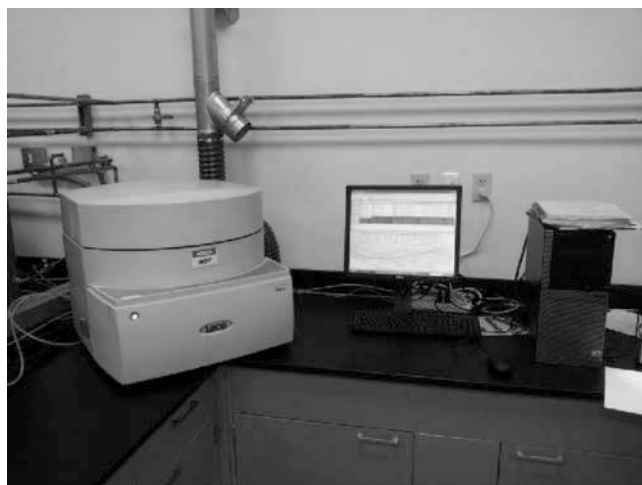
Figure 2: TGA701 with desktop computer interface.
