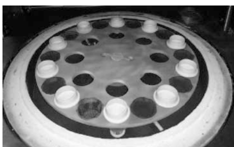
Figure 17: Blank Crucible Separation used for the routine testing procedures. Samples are placed in the dark nichrome crucibles.
