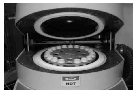
Figure 4: TGA carousel loaded with ceramic crucibles.
