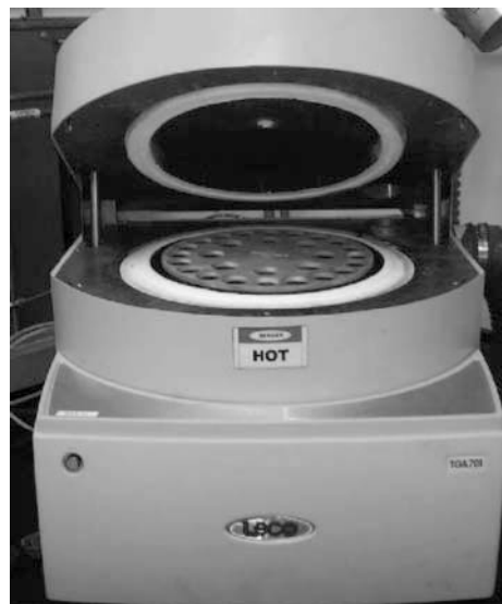
Figure 3: TGA with open lid and empty sample carousel.
