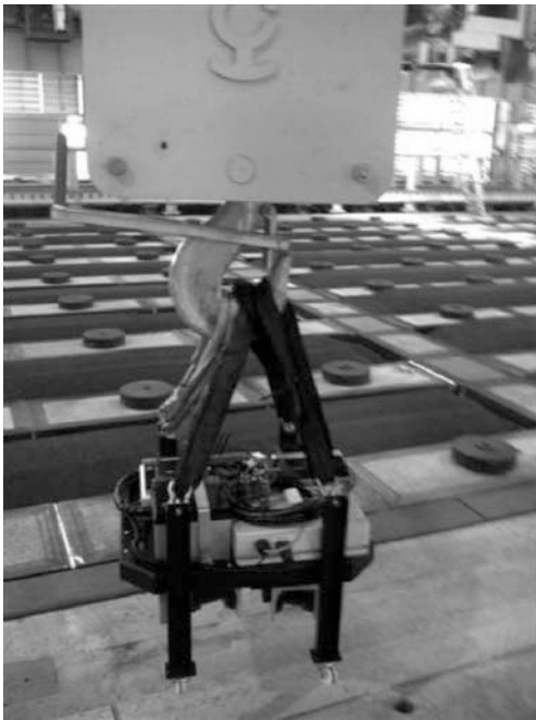
Figure 1: The sensor rig attached to a crane in the CBF. The lidar sensors can be seen under the rig’s frame with the control and logging PC, batteries and cabling above it.
