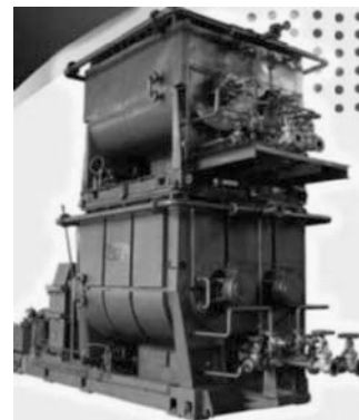
Figure 4: Picture of double layer batch mixer
