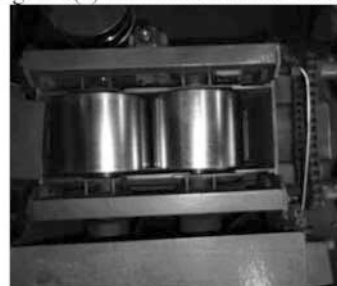
Figure 4(d) Petrocoque's Roller Crusher
