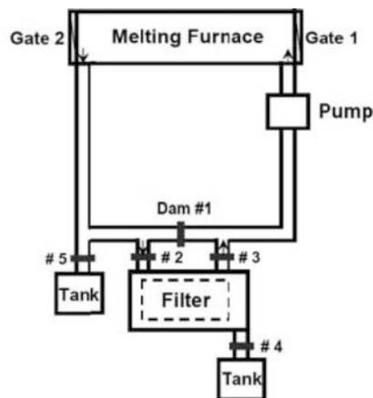
Figure 1 The schematic top view of the filtration loop
