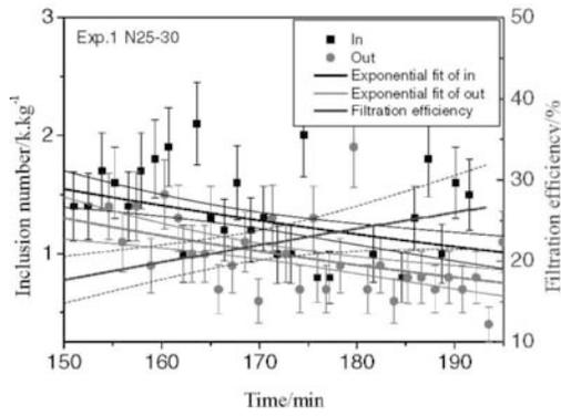
Figure 7 The inclusion number (density) and filtration efficiency for inclusions 25-30 μm in Exp.1 using an Al<sub>2</sub>O<sub>3</sub> filter
