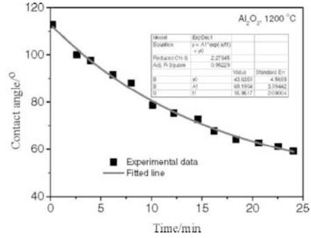
Figure 4 Contact angle at 1200°C for the Al<sub>2</sub>O<sub>3</sub> industrial filter
