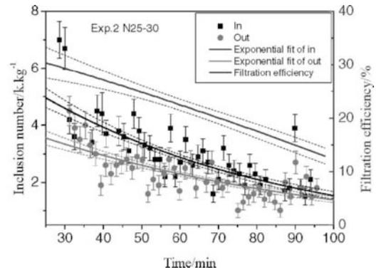
Figure 8 The inclusion number (density) and filtration efficiency for inclusions 25-30 μm in Exp.2 using a SiC filter
