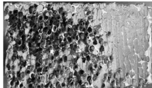
Figure 13 Cross sectional view of the SiC spent filter in Exp.4
