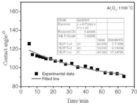
Figure 3 Contact angle at 1100°C for the Al<sub>2</sub>O<sub>3</sub> industrial filter
