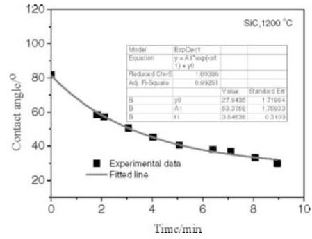
Figure 6 Contact angle at 1200°C for the SiC industrial filter
