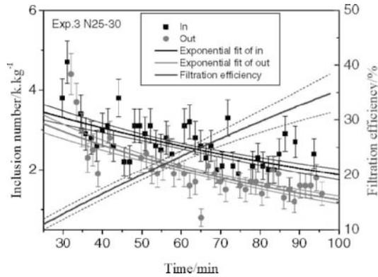
Figure 9 The inclusion number (density) and filtration efficiency for inclusions 25-30  $\mu\text{m}$  in Exp.3 using an  $\text{Al}_2\text{O}_3$  filter
