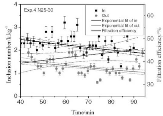
Figure 10 The inclusion number (density) and filtration efficiency for inclusions 25-30  $\mu\text{m}$  in Exp.4 using a SiC filter
