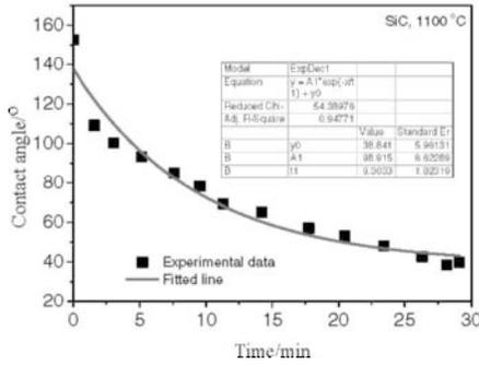
Figure 5 Contact angle at 1200°C the SiC industrial filter
