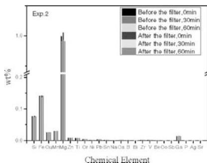
Figure 2 The content of alloying elements before and after the filter in Exp.2 using a SiC filter
