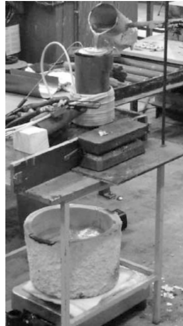
Figure 2. Experimental apparatus for the flow filtration experiments, showing aluminum metal being added continuously via a ladle and discharging into a receiving vessel placed on a weightometer [5].
