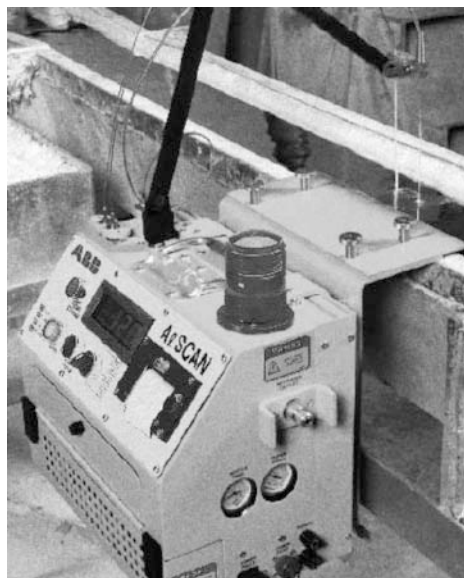
Figure1. Alscan testing H 2 levels
