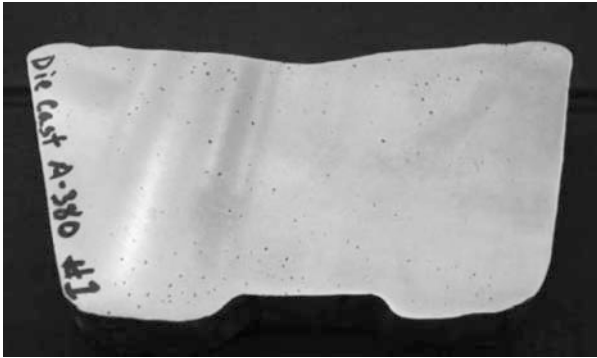
Figure 16. Cross section of 'gassy' ingot
