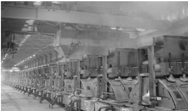
Figure 2 – Manual filling of overhead pot bins
