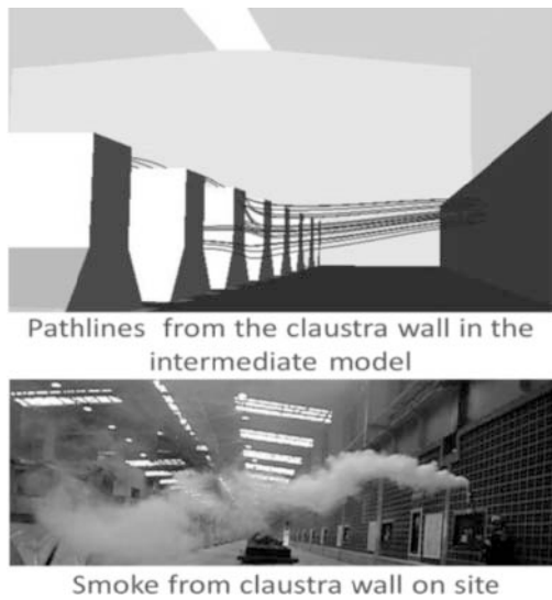
Figure 7 : Comparison between smoke test and modelling with the intermediate model
