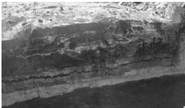
Figure 6. Cathode panel heave and cathode block destruction on cell failed in 5 days after metal restart.
