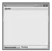
Figure 13-1. A GUI window with a BackgroundWorker reporting progress percentage
