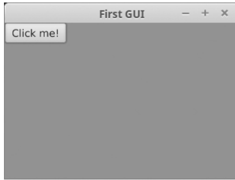
FIGURE 11.1: This is the window that pops up running JustButton.scala . There is a single button in a 300 by 200 pixel scene. Note that the button is, by default, in the top left corner.
