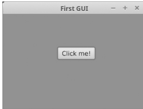
FIGURE 11.2: This is the window that pops up when you run MovedButton.scala . Notice that the button has been moved so that it is roughly centered in our 300 by 200 pixel window.
