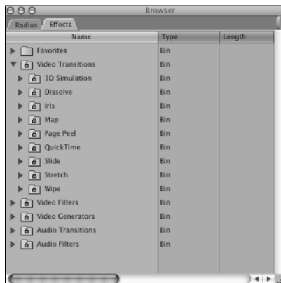
Figure 6-5: Click the Browser's Effects tab to see all the Final Cut Pro filters, transitions, and generators.
