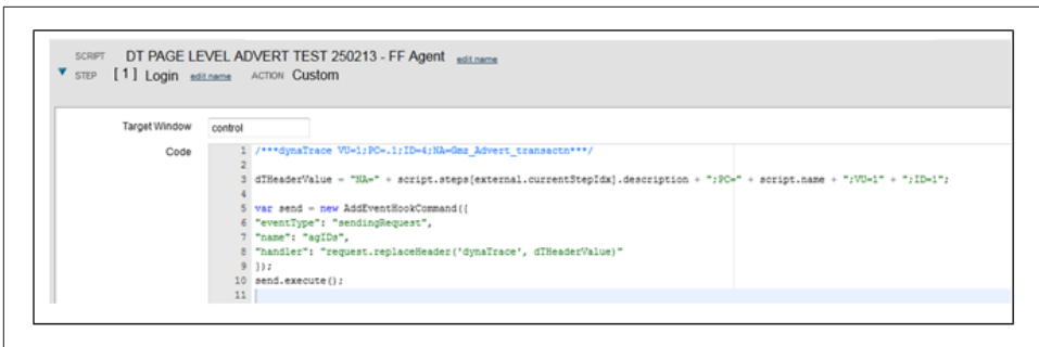
Figure 8-1. Inserting a header flag to identify synthetic test traffic to an APM tool (in this example Gomez SaaS/Compuware dynaTrace)
