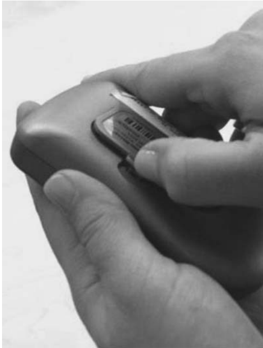
FIGURE 12.6 A test participant struggles to open the battery compartment of a medical device using her fingernail.
