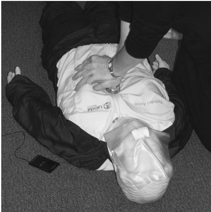
FIGURE 17.1 The need to protect human subjects from harm calls for the use of a Resusci Anne® or another mannequin to evaluate the performance of a CPR assist device, which guides users to compress the victim's chest an appropriate amount and at the right pace.
