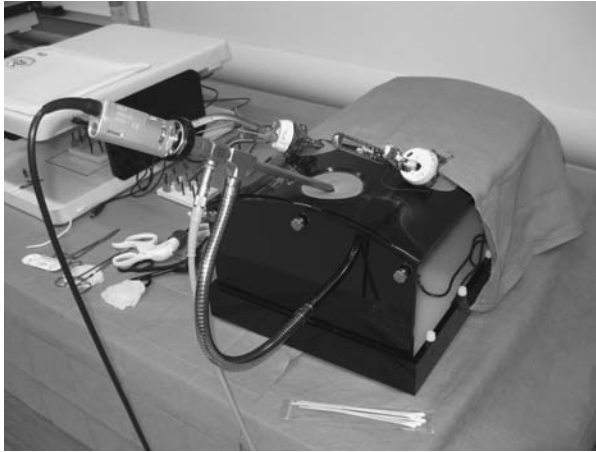
FIGURE 10.6 (See color insert following page 202.) A simulation of the human pelvic region used for training clinicians to use minimally invasive surgical tools. Photo courtesy of Vanderbilt University School of Medicine.
