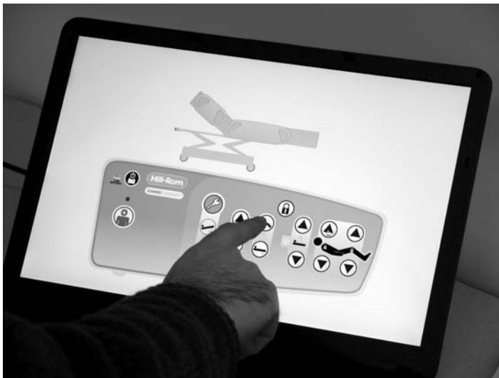
FIGURE 10.18 (See color insert following page 202.) A computer-based simulation of a hospital bed control panel displayed on a touch screen computer.
