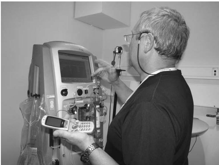
FIGURE 10.1 (See color insert following page 202.) A usability test participant is distracted by a phone call while using a dialysis machine.
