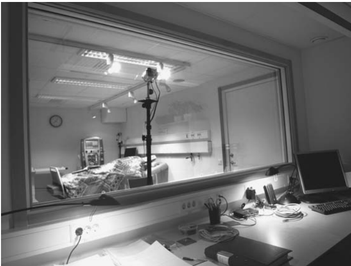
FIGURE 1.1 (See color insert following page 202.) A conventional usability testing lab equipped with a one-way mirror.
