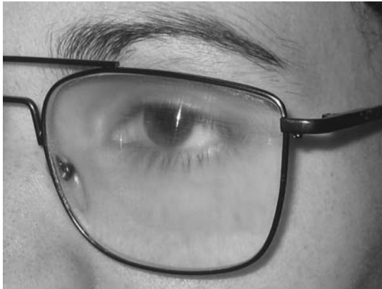
FIGURE 10.12 Having test participants wear a pair of glasses smeared (on the outside) with a harmless substance (e.g., Vaseline®) is a “quick-and-dirty” way to create blurry vision.
