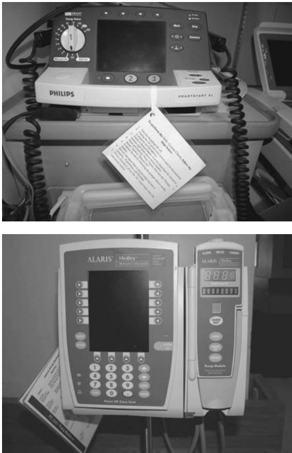
FIGURE 12.10 Quick reference cards attached to a defibrillator (top) and infusion pump (bottom).
