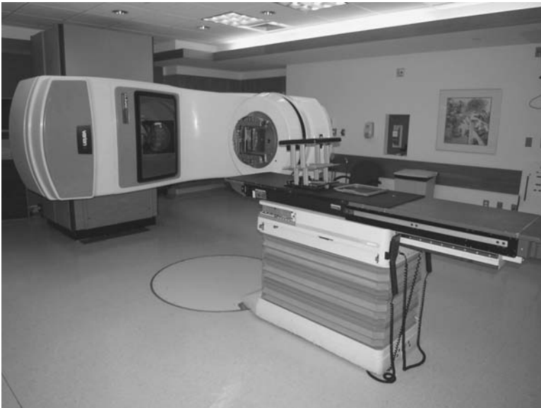
FIGURE 9.10 (See color insert following page 202.) This immovable radiation therapy machine would require on-site testing as opposed to testing in a usability test laboratory.
