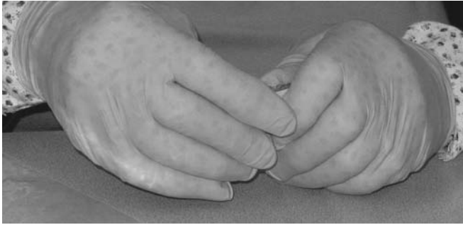
FIGURE 10.14 A test participant wears two pairs of gloves (cotton and protective) to simulate dexterity and sensation limitations.
