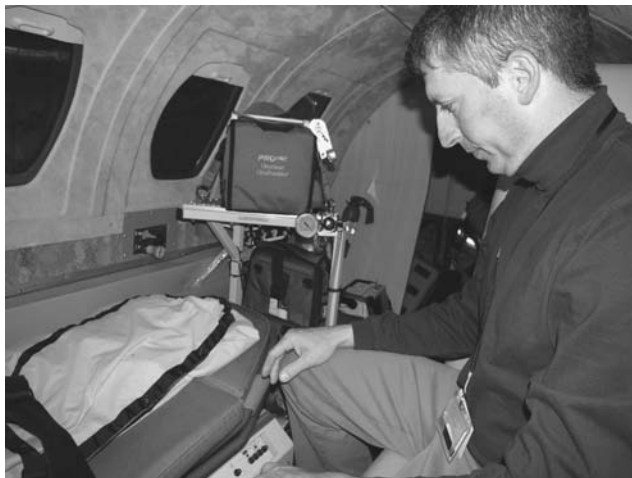
FIGURE 9.4 Conducting a usability test of a medical device in an air ambulance (small jet).
