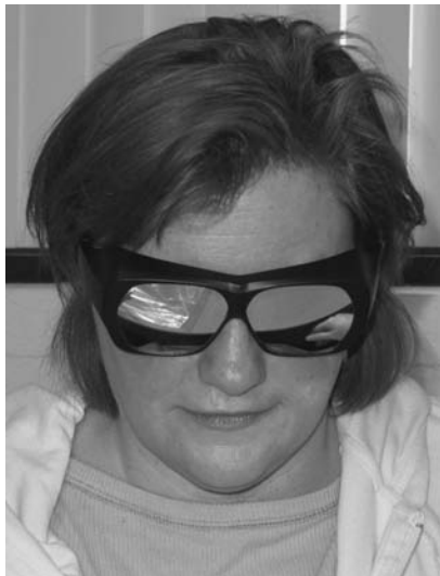
FIGURE 10.16 (See color insert following page 202.) A test participant wears Variantor™ glasses to simulate color-impaired vision.
