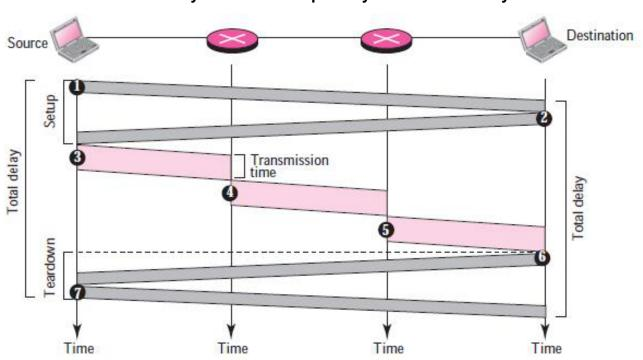
Total delay=3T+3τ+setup delay+teardown delay
