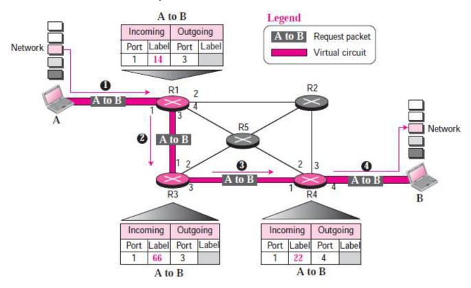
**Acknowledgment:** A special frame, called the acknowledgment frame, completes the entries in the switching tables. The next figure shows the process.
