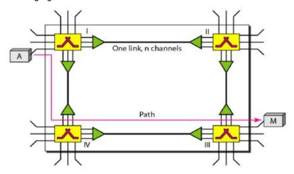
System A needs to connect to system M, it sends a setup request that includes the address of system M, to switch I.
