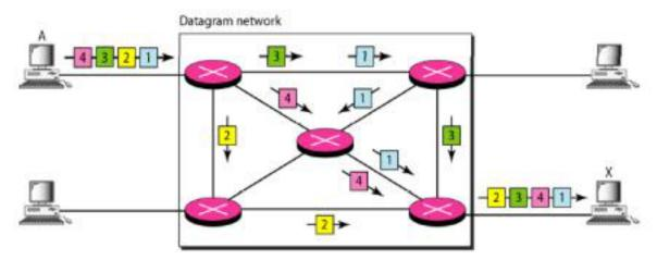
We can note that all four packets (or datagrams) belong to the same message, but may travel different paths to reach their destination. This approach can cause the datagrams of a transmission to arrive at their destination out of order with different delays between the packets. Packets may also be lost or dropped because of a lack of resources. The datagram networks are sometimes referred to as connectionless networks. There are no setup or teardown phases.
