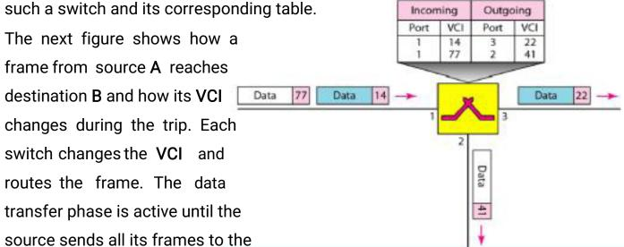
destination. The procedure at the switch is the same for each frame of a message.
