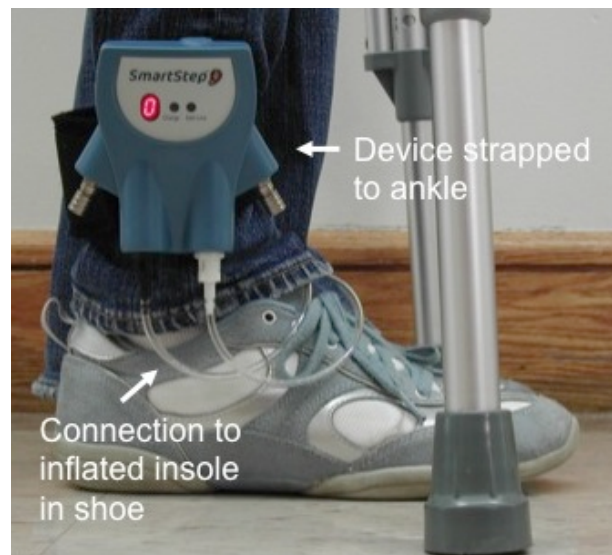
Figure 1. Labeled diagram of the SmartStep weight-monitoring device (Andante Medical Devices, Ltd, Omer, Israel).
