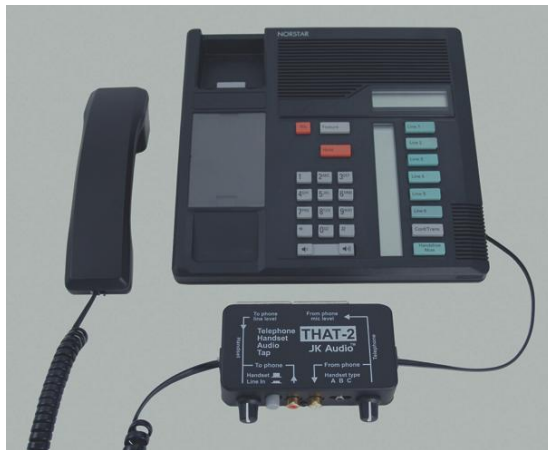
Figure 2.6 This device ( bottom center ) lets you connect the phone and the IVR system to your logging and/or recording computer.
