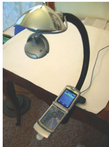
Figure 2.5 A do-it-yourself solution for testing a mobile device can be built using locally available parts.
