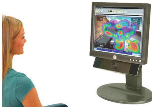
Figure 2.2 EyeTech's eye-tracking device attached to the participant's monitor displays the results with a heat map.
