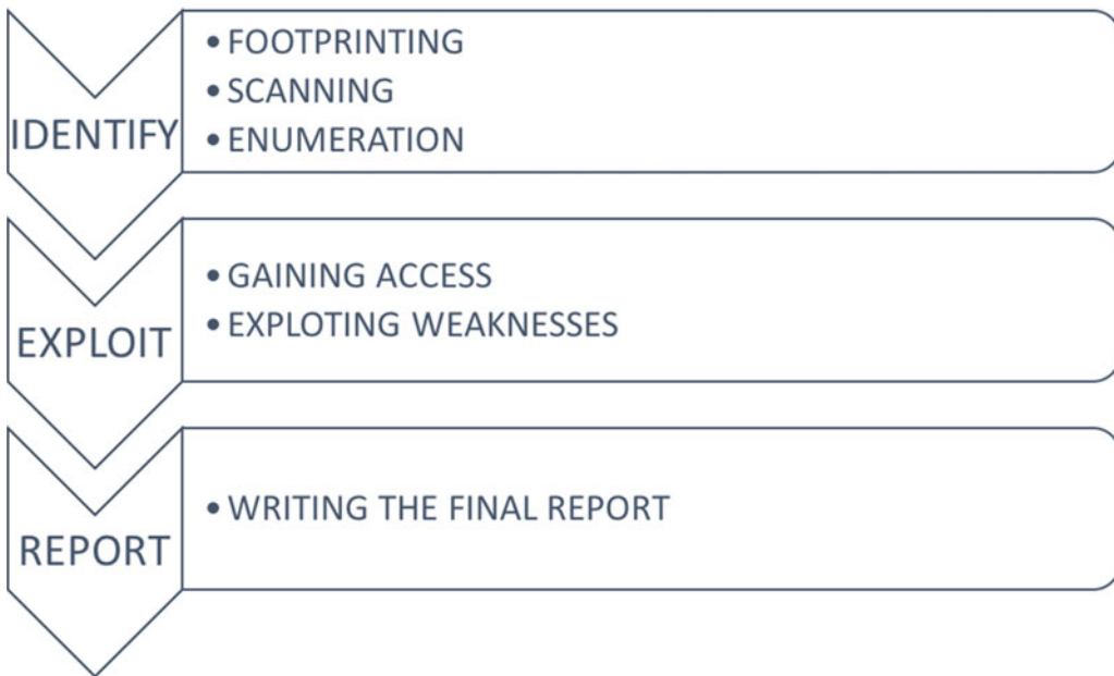
Figure 5-2. The layered approach by example applied to a black box security test
