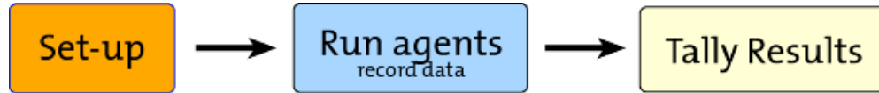
Fig. 11-3: The overall test is divided into three parts. The Set-up part describes the test environment, number of concurrently running test agents, and behavior of each agent based on a user archetype. The second part actually runs the agents and records the results to a log file. The third part analyzes the recorded results and presents the findings.
