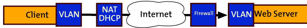
Fig 10-3: Software at the client and server devices to encrypt data communicated over a Web infrastructure forms a Virtual Private Network (VPN.)
