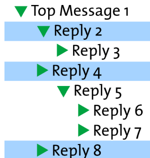
Figure 8-8: Reply messages 2, 4 and 8 are branches off the Top Message. While the discussion group is being created the agent must remember the branch locations to know how to handle commands to create new branches.
