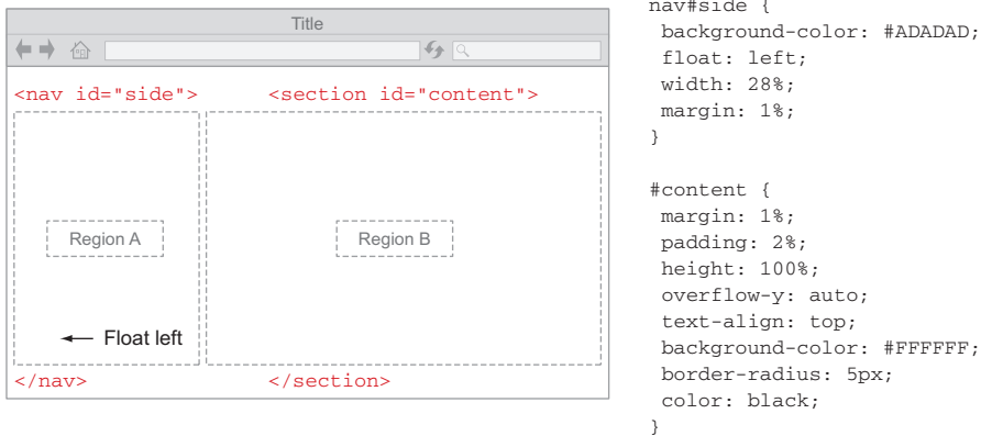
Figure 5.4 CSS is used to define the physical attributes of the regions in your layout, as well as to define their relationship with other regions in the UI.
