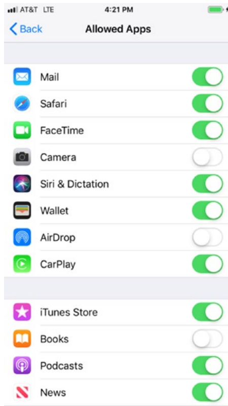
Figure 3-5. Restricting apps which can be used on this iOS device
