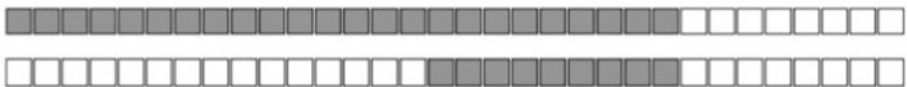
Figure 5-12. The top is the current match's mask (0xFFFFF00), and the bottom is a Grenadier mask (0x0000FF00)
