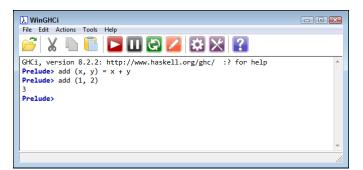
FIGURE 4-1: Create and use a new function named add.
