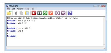
FIGURE 4-4: Currying makes creating new functions easier. Interestingly enough, you can convert between curried and non-curried versions of a function as needed using the built-in curry and uncurry functions. Try it with add by typing **uadd = uncurry add** and pressing Enter. To prove to yourself that uadd is indeed the non-curried form of add, type **uadd 1 2** and press Enter. You see the error shown in Figure 4-5.
