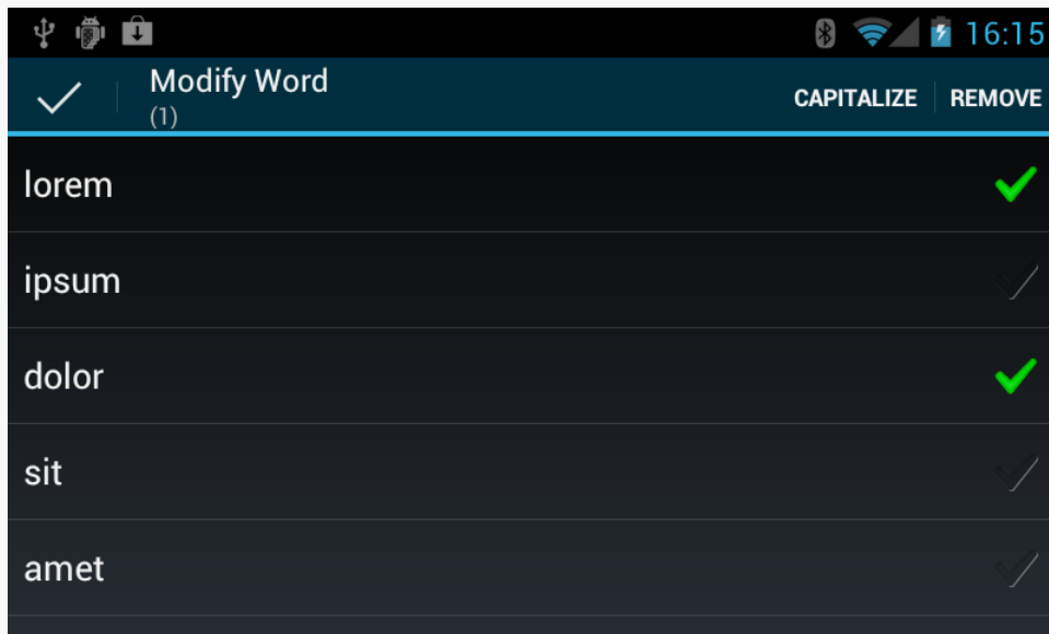
Figure 248: The ActionModeMC sample on a phone, using a split action bar, in landscape orientation
