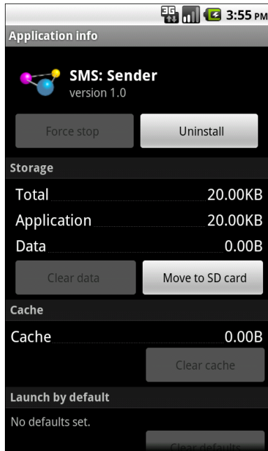
Figure 98. An application, installed on the on-board flash but movable to the SD card
