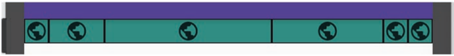
Figure 6-22. Expandeds have flex property to control how much extra space each gets
