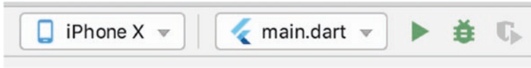
Figure 2-7. The Play and Debug buttons are at the top in Android Studio
