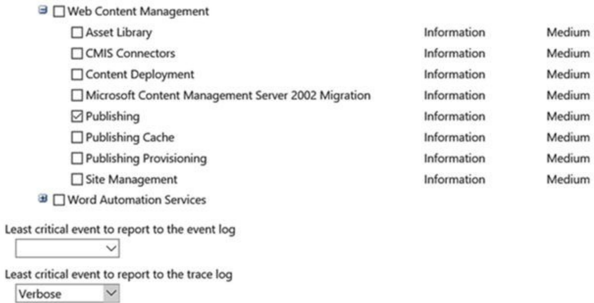
Figure 18-5. Adjusting the verbosity of an Area
