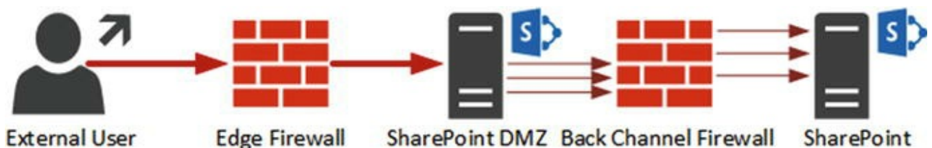
Figure 4-5. SharePoint in the DMZ with multiple ports open in the Back Channel Firewall
