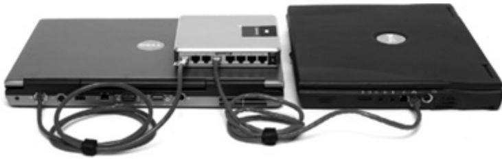
Figure 22-10 A switch connected by UTP cable to two PCs
