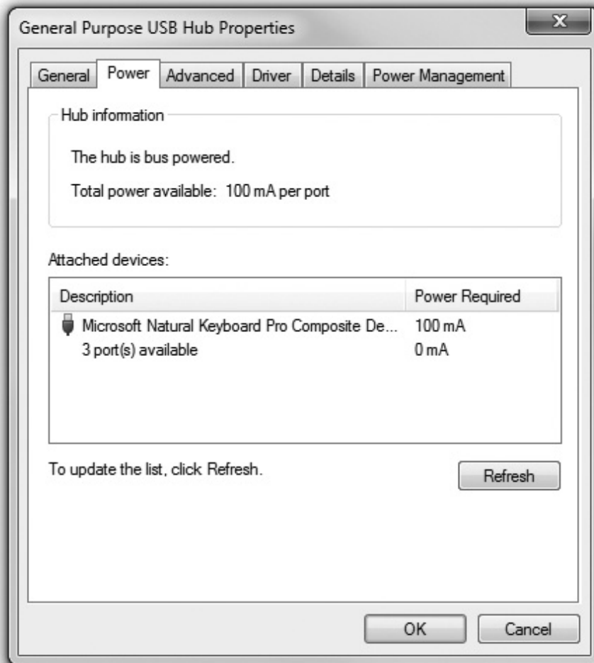
Figure 20-14 General purpose bus-powered hub
