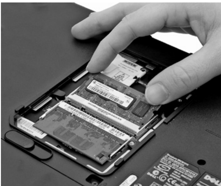
Figure 26-47 Releasing the RAM
