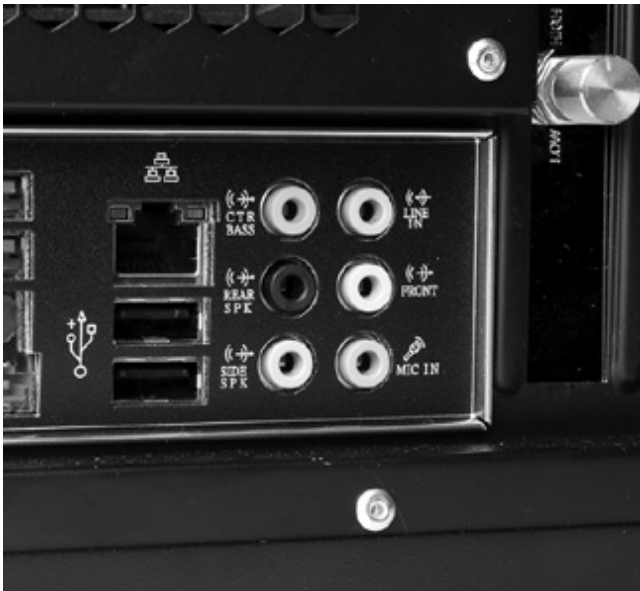
Figure 3-22 Typical bank of 1/8-inch audio jacks
