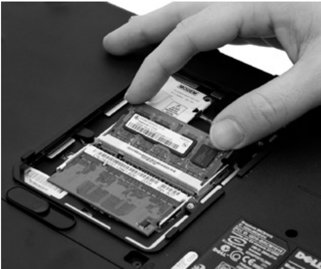
Figure 7-40 Snapping in a SO-DIMM
