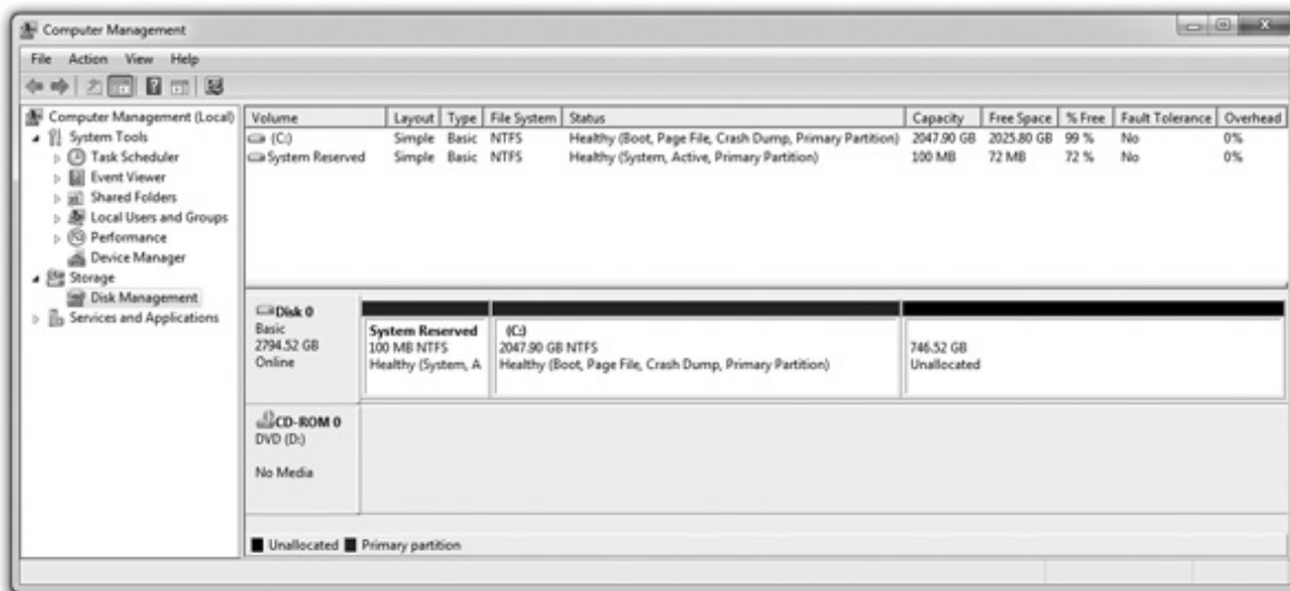
Figure 8-33 Here's what happens when you install Windows 7 on a greater-than-2.2-TB drive using regular BIOS.
