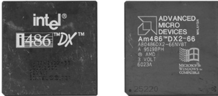
Figure 6-19 Identical Intel and AMD 486 CPUs from the early 1990s
