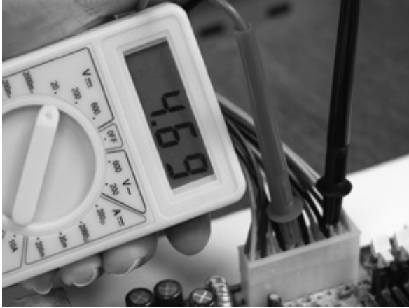
Figure 10-38 Testing one of the 5-V DC connections
