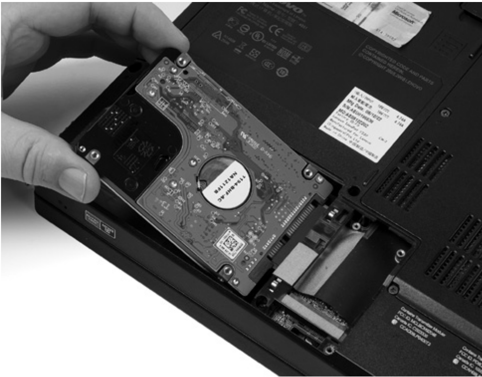
Figure 26-50 Inserting a replacement drive
