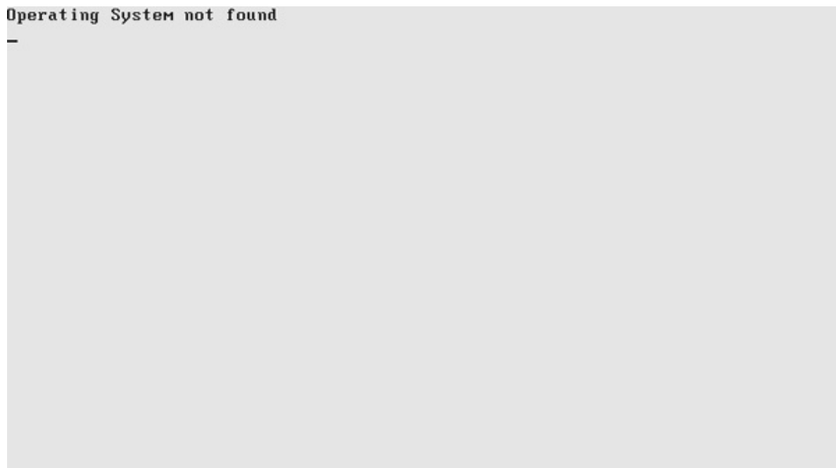
Figure 19-1 If you see this screen, the problem is with hardware. Windows hasn't even started trying to boot.
