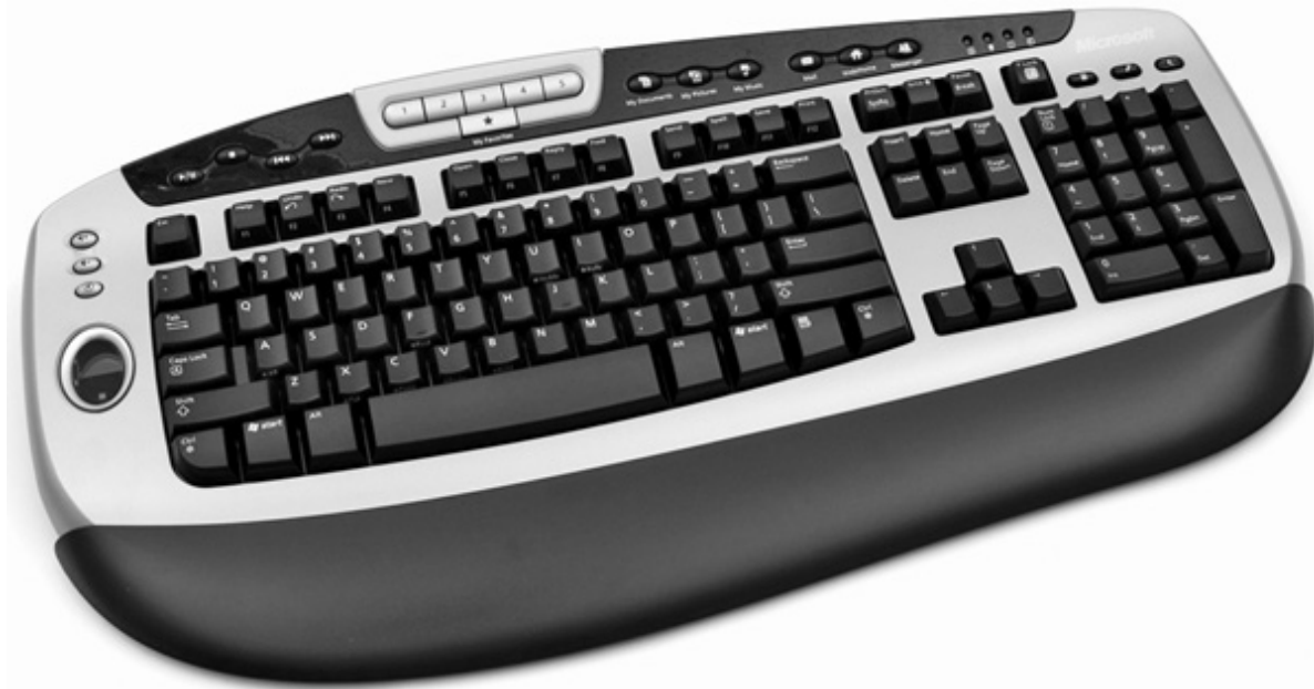
Figure 29-11 Microsoft keyboard with fingerprint accessibility
