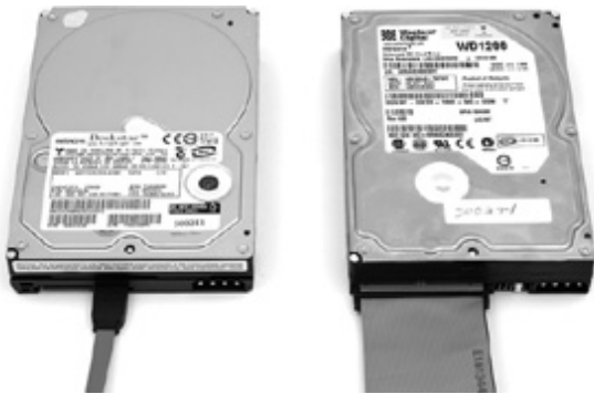
Figure 3-43 SATA and PATA drives showing data connectors
