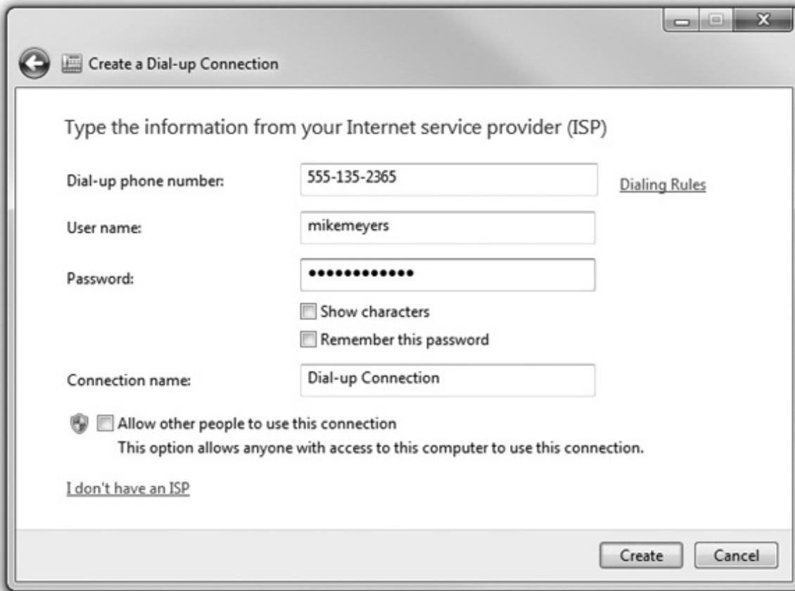
Figure 24-18 Creating a dial-up connection in Windows 7
