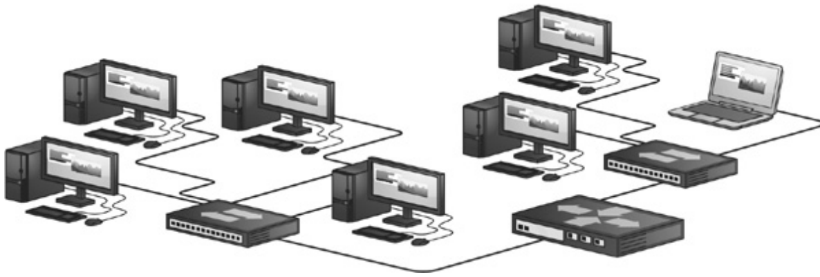
Figure 5-16 Two broadcast domains connected by a router—a WAN
