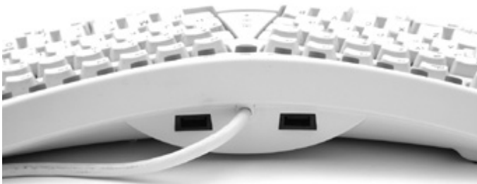
Figure 20-11 USB keyboard with built-in hub
