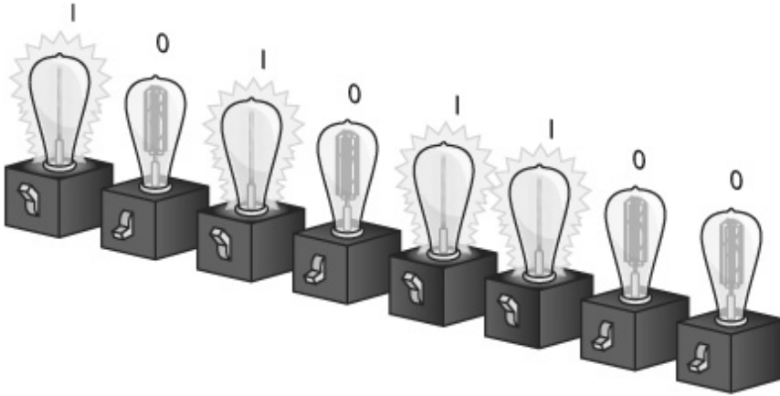
Figure 6-5 Here "1" means on, "0" means off.
