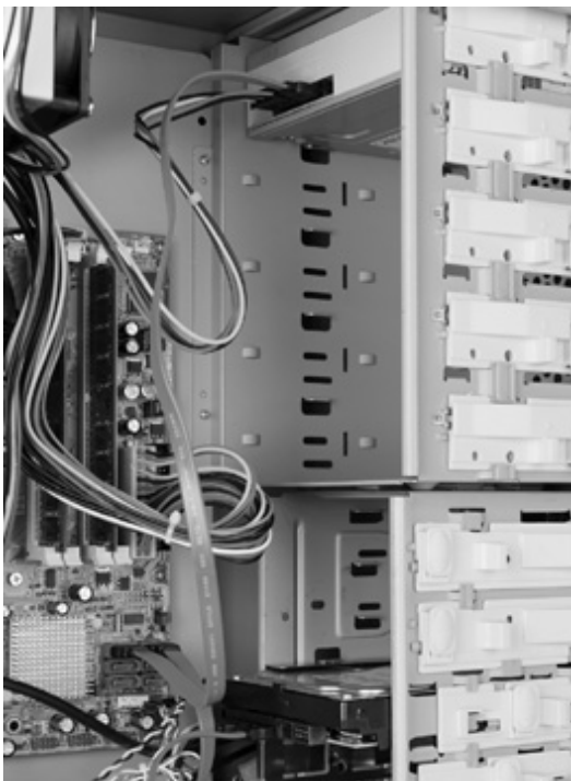
Figure 13-30 Typical DVD installation
