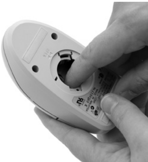
Figure 20-27 Cleaning the rollers on a ball mouse
