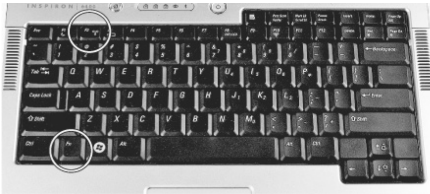
Figure 26-16 Laptop keyboard showing Function (FN) key that enables you to access additional key options, as on the F2 key
