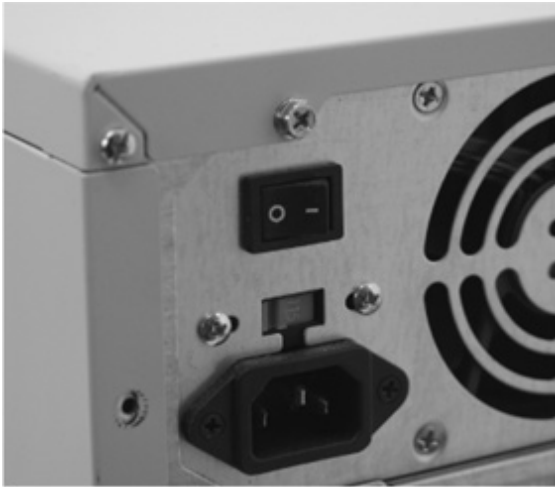
Figure 10-3 Back of fixed-input power supply, showing typical switches and power connection
