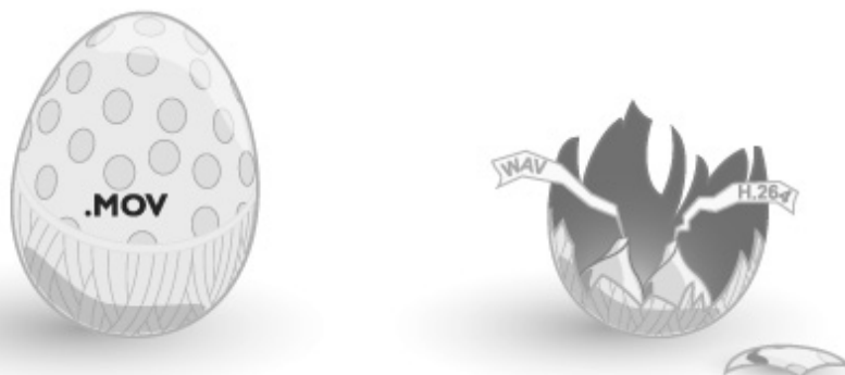
Figure 25-32 A standard container file holds multiple tracks, each encoded separately.
