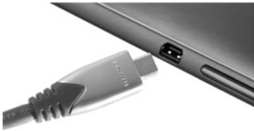
Figure 27-25 Micro-HDMI port and connector
