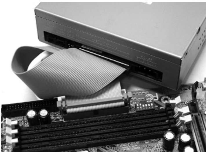
Figure 11-15 ATAPI CD-RW drive attached to a motherboard via a standard 40-pin ribbon cable
