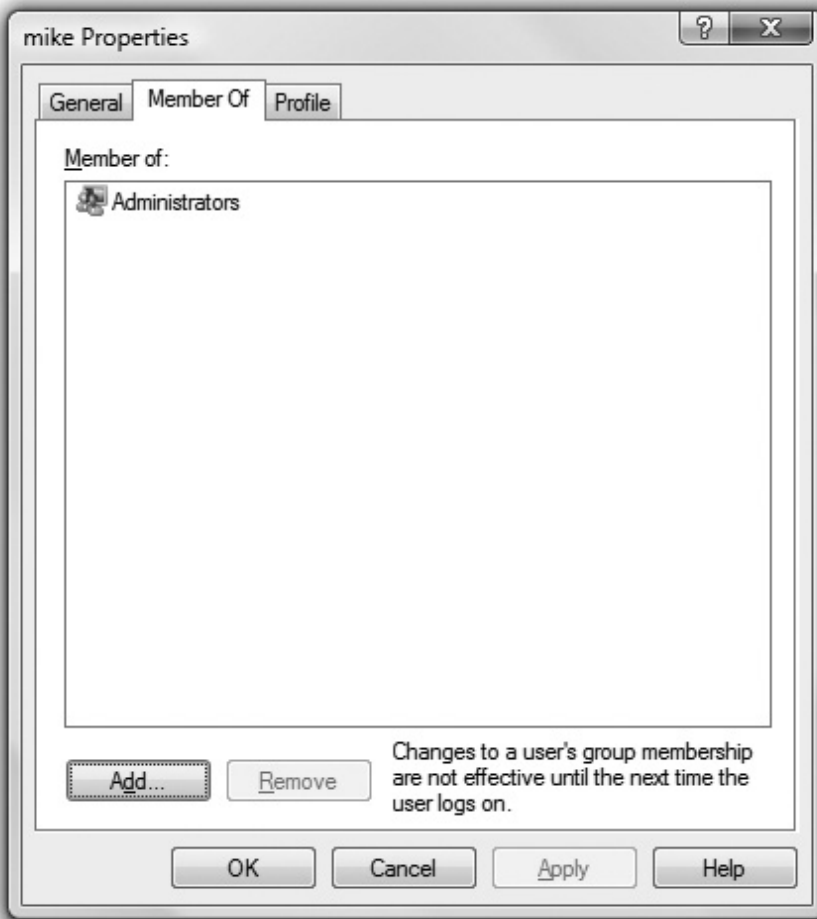
Figure 16-20 Properties dialog box of a user account, where you can change group memberships for that account
