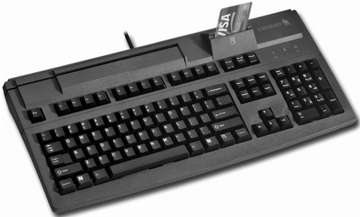
Figure 29-7 Keyboard-mounted smart card reader being used for a commercial application (photo courtesy of Cherry Corp.)
