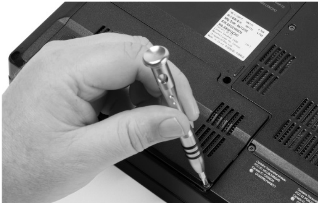
Figure 26-49 Removing the drive compartment cover
