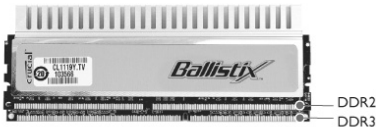
Figure 7-17 DDR2 DIMM on top of a DDR3 DIMM
