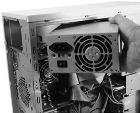
Figure 10-28 Removing power supply from system unit
