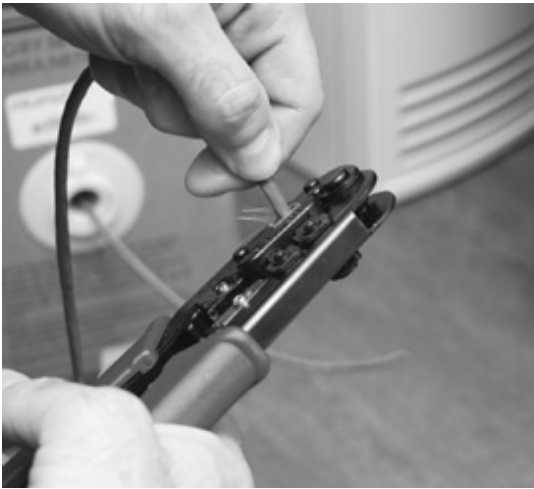
Figure 22-26 Crimping the cable
