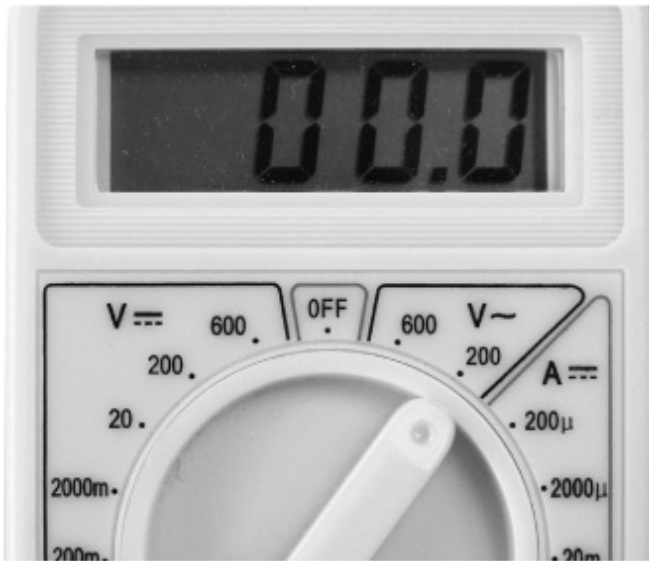
Figure 10-6 Multimeter featuring DC and AC symbols
