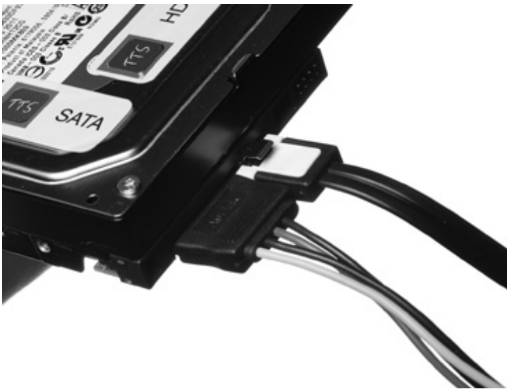
Figure 11-43 Properly connected SATA cable
