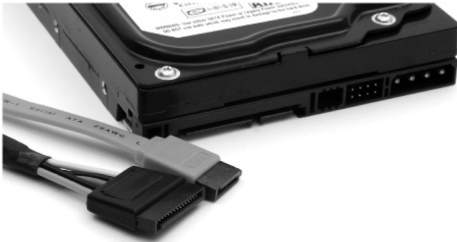
Figure 11-20 SATA hard disk power (left) and data (right) cables
