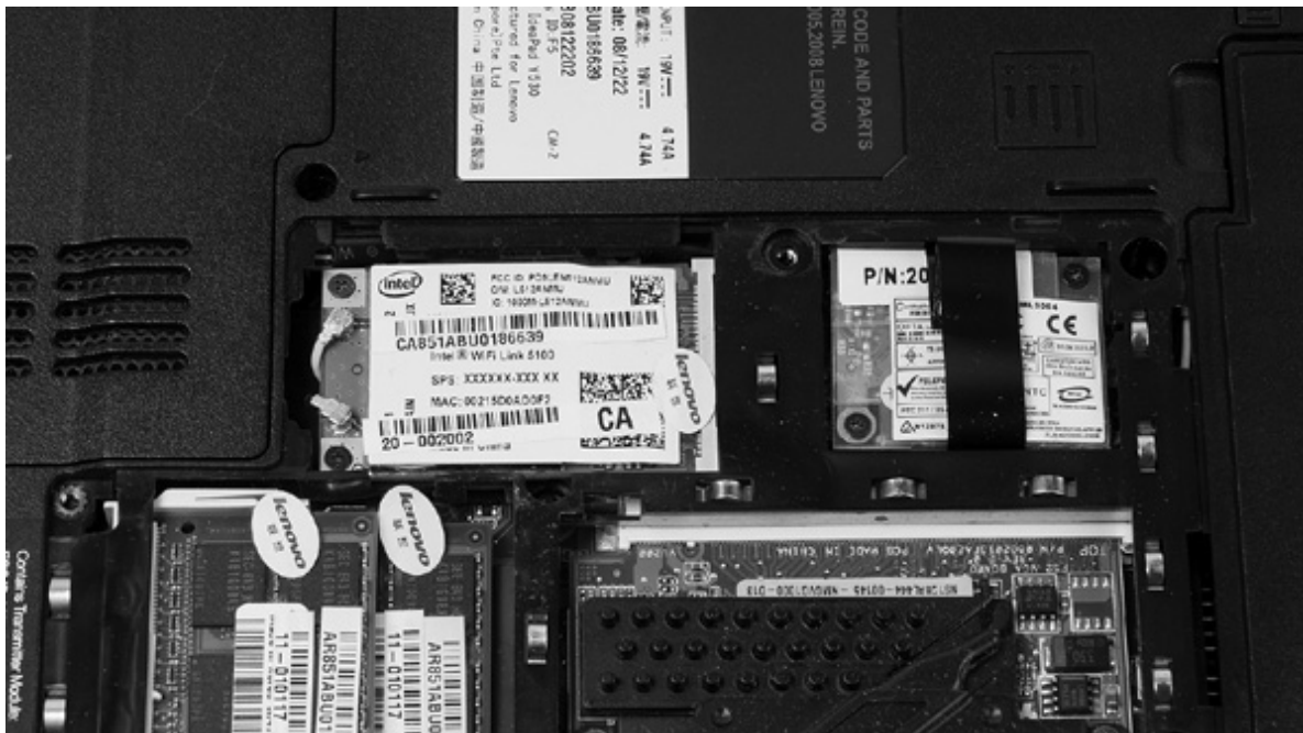
Figure 26-52 Mini-PCIe expansion slot on laptop
