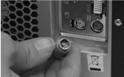
Figure 3-26 Mouse with mini-DIN connection
