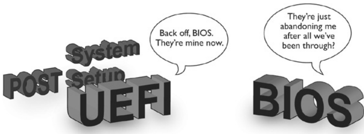
Figure 8-36 POST and system setup are still here.
