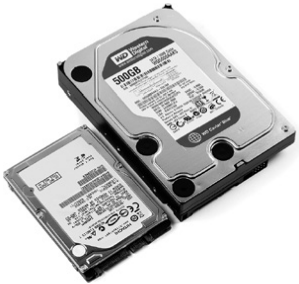
Figure 26-48 The 2.5-inch and 3.5-inch drives are mostly the same.
