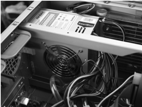
Figure 10-1 Typical power supply mounted inside the PC system unit
