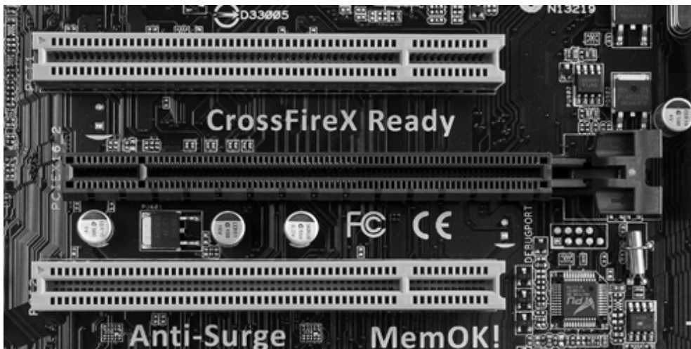
Figure 9-30 PCIe \times 16 slot (center) with PCI slots (top and bottom)
