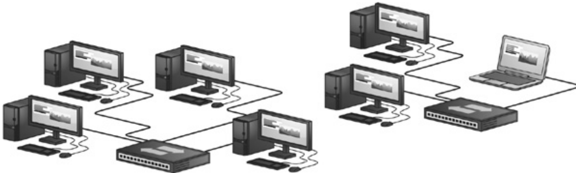
Figure 5-15 Two broadcast domains—two separate LANs
