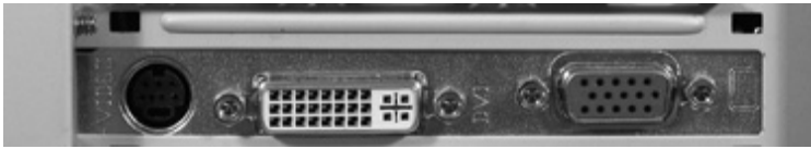
Figure 3-20 Video card with (from left to right) S-Video, DVI, and VGA ports
