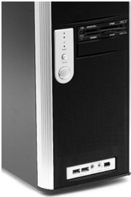
Figure 9-47 Case with both front-mounted ports and an add-on flash memory card reader
