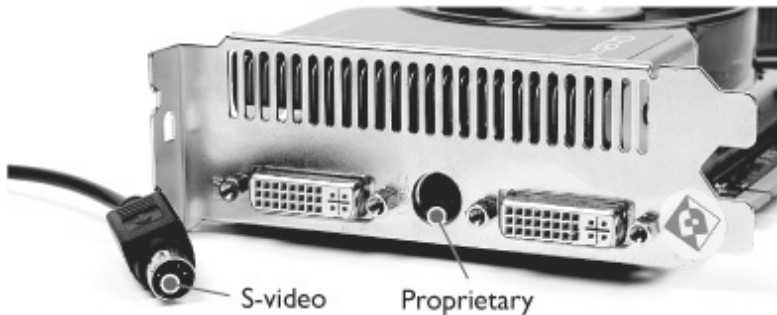
Figure 21-45 S-video and proprietary round connectors
