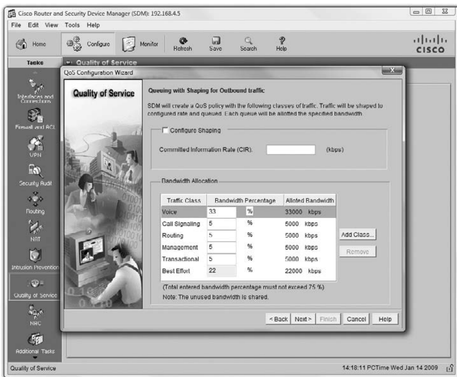
Figure 12-27 QoS configuration on a router
