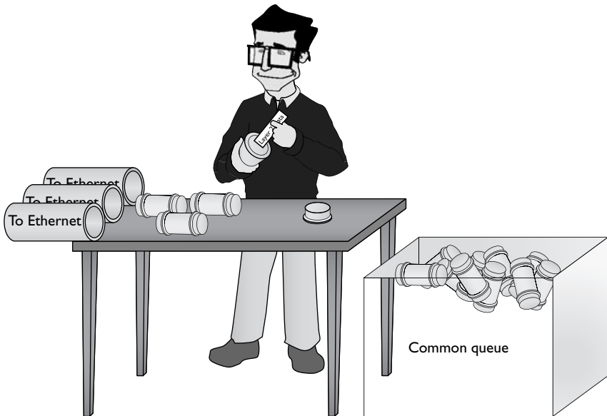
Figure 8-6 All incoming packets stripped of Layer 2 data and dropped into a common queue
