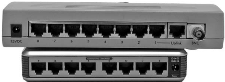
Figure 4-25 Hub (top) and switch (bottom) comparison
