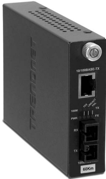
Figure 4-14 Typical copper-to-fiber Ethernet media converter (photo courtesy of TRENDnet)
