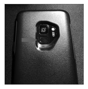
A phone fingerprint sensor on a Samsung Galaxy S9 in an Otterbox case. Some phones have the reader on the front, while others, like the S9, have it on the back.
