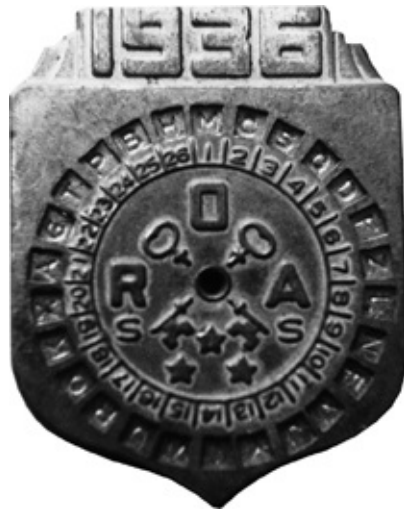
Figure 32 Captain Midnight's Code-o-Graph, which enciphers each plaintext letter (outer disk) as a number (inner disk), rather than a letter.
