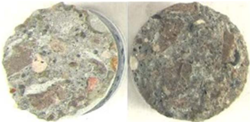
Figure 6.9 Failures of concrete substrate.
