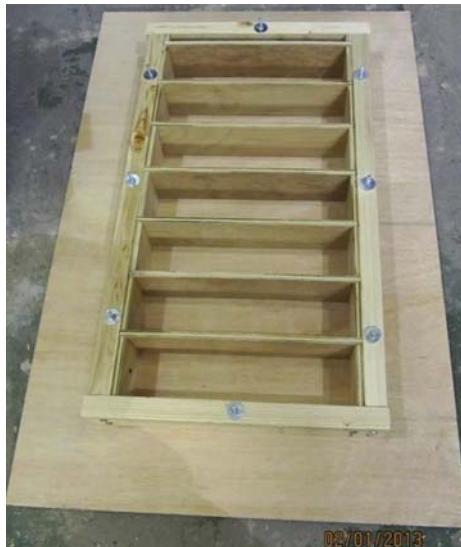
Figure 6.1 Reusable plywood mold for seven specimens.
