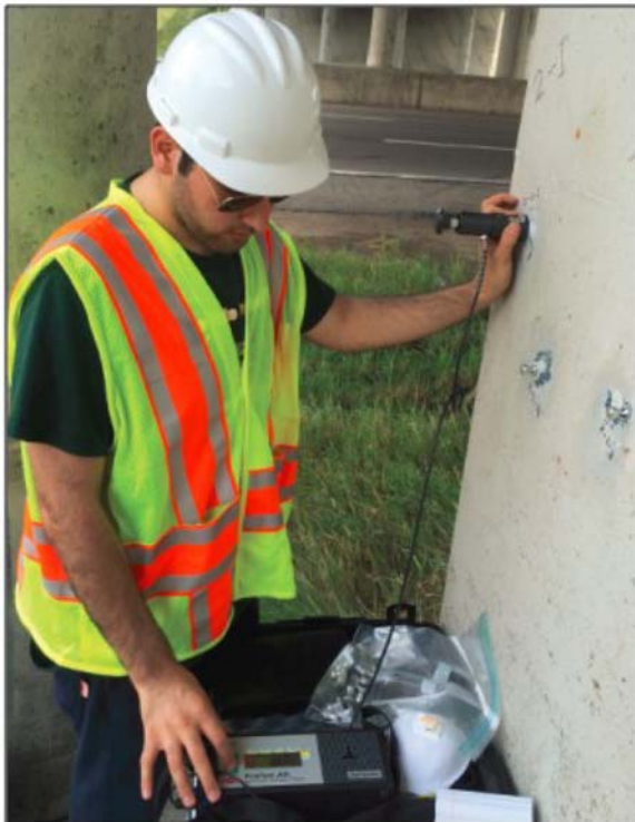
Figure 7.3 Adhesive bond testing on as-built structure.
