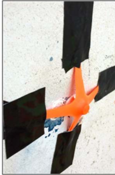
Figure 7.1 Test dolly secured with rubber membrane.
