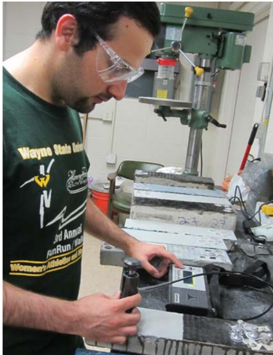
Figure 6.6 Pull-off test underway.
