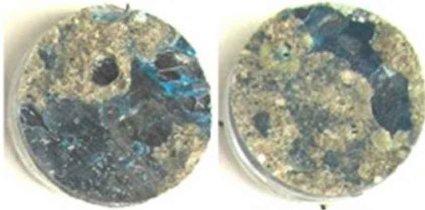
Figure 6.10 Mixed failures through FRP resin (bond failure) and concrete substrate.
