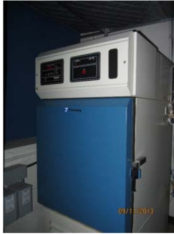
Figure 6.3 Tenney environmental chamber.
