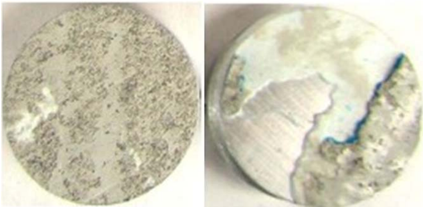
Figure 6.7 Bond failures between dolly and FRP.
