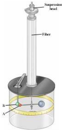
Figure 23.6 Coulomb's torsion balance, used to establish the inverse-square law for the electric force between two charges.
