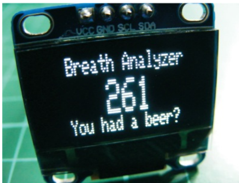
FIGURE 19-2: 128×64 OLED monochrome screen. When the MQ3 reads the value, the Arduino sends a message to the OLED screen indicating whether or not alcohol has been detected.
