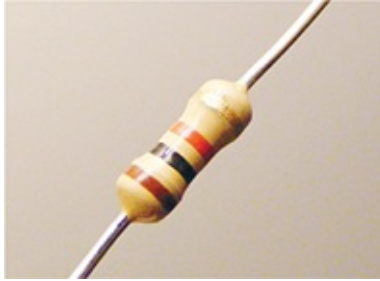
FIGURE B-1: A four-band resistor
