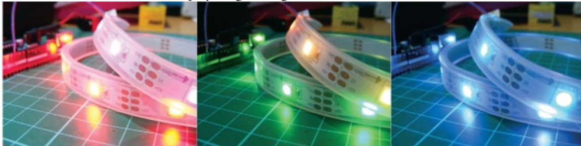
FIGURE 6-2: RGB LED strip cycling through the colors of the rainbow
