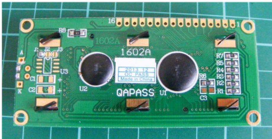
FIGURE 16-2: The reverse side of the LCD screen
