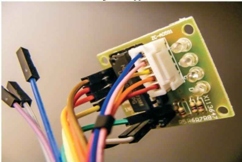
FIGURE 11-2: Connecting the stepper to the driver board
