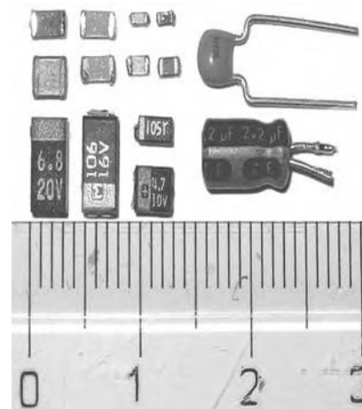
FIG. 1-12. Chip and ceramic capacitors. (Courtesy of Wikipedia)
