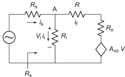
$$i_s = i_i + i_f = \frac{v_i}{R_i} + \frac{v_i - A_{vo} v_i}{R + R_o}$$
