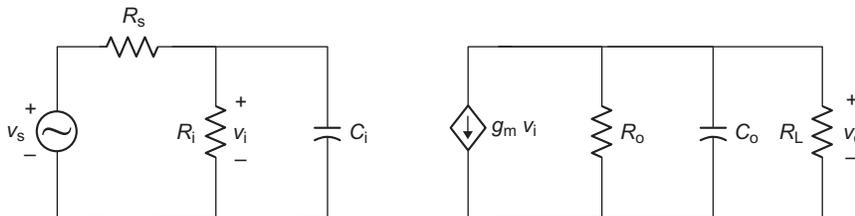
$$v_o = -g_m v_i \left( R_o \parallel R_L \parallel \frac{1}{sC_o} \right)$$
