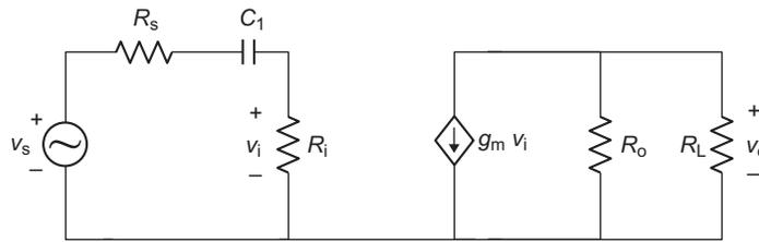
Low-frequency equivalent circuit
