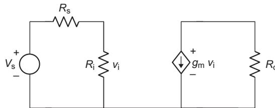
$$v_o = -g_m v_i R_o = -\frac{g_m R_i \cdot R_o}{R_s + R_i} v_s$$
