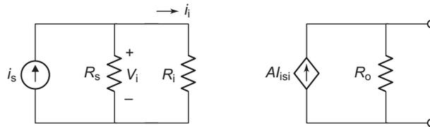
(a) Output resistance =  $\frac{\text{open-circuit voltage}}{\text{short-circuit current}}$
