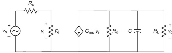
$$\begin{aligned} \text{(a)} \quad v_o &= -G_{ms} v_i \left( R_o \parallel \frac{1}{sC} \parallel R_L \right) \\ &= -20 \times 10^{-3} v_i \left( 980 \parallel \frac{1}{sC} \right) \end{aligned} \quad \text{(i)}$$
